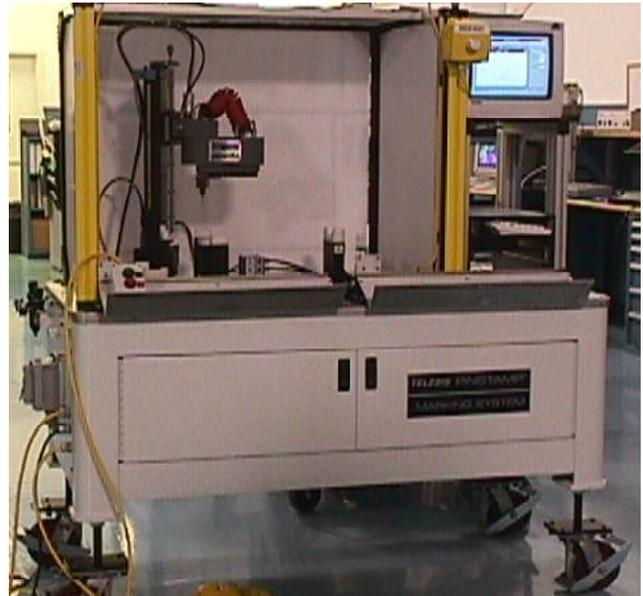
**An integrated TMP6100/700 Marking System combines parts nests and sensors with custom software to match parts and patterns. Valid print data is then sent to the barcode label printer. The system, including automatic Z-axis mounting post, is mounted on a custom wheeled base.**
